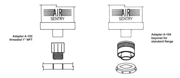
Air Sentry Breathers use a three-stage filtration design to ensure optimum protection by removing water vapor and solid contaminants before they enter the fluid system.
