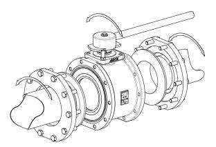
Loose body flanges make it possible to install the valve without aligning of the welded end connections. After installation the valve can rotate on 360° for the desired orientation.
